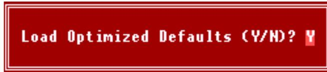
Pressing Y loads the default factory settings for optimal system performance.
