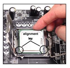
8. Cover the load plate onto the package.
