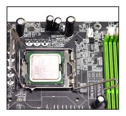
After confirming the CPU direction for correct mating, put down the CPU in the socket housing frame. Be sure to grasp on the edge of the CPU base. Note that the alignment keys are matched.
