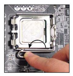
11. Press the four hooks down to fasten the cooler. Then rotate the locking switch (refer to the correct direction marked on it) to lock the hooks.
