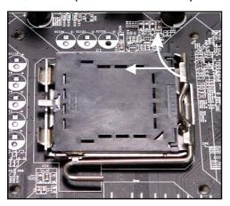
2. Remove the cap from lever hinge side (as the arrow shows).
