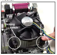
10. Align the holes on the mainboard with the heatsink. Push down the cooler until its four clips get wedged into the holes of the mainboard.
