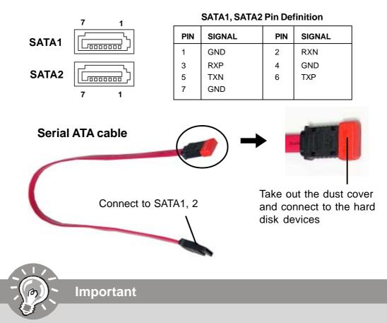
Please do not fold the Serial ATA cable into 90-degree angle. Otherwise, data loss may occur during transmission.
